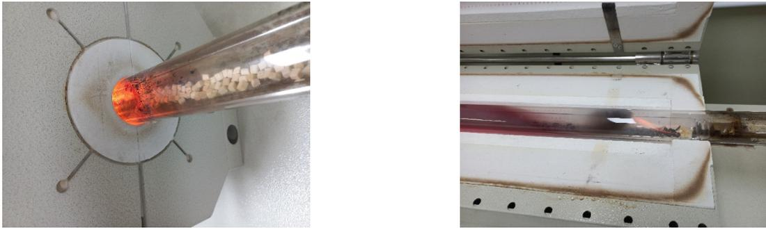
Figure 3. Typical fire flames of wood cubes: Inlet part (Left) and inside (Right) of the furnace.
