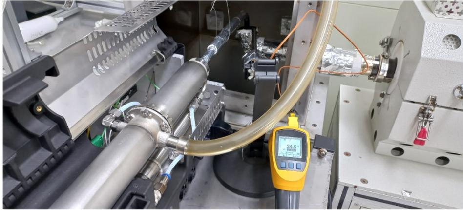
Figure 2. Photo of the direct sampling of particles at the exit of the furnace.
