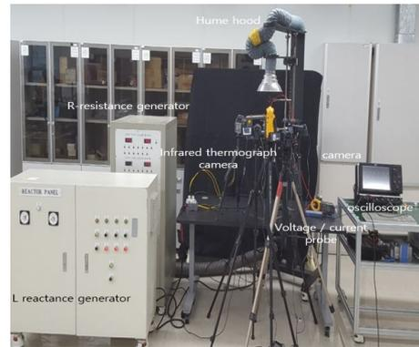
Figure 2. The composition of the basic experiment.
